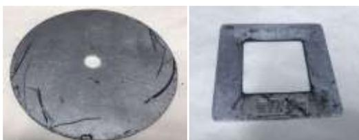
Gambar 5 Mal titi Pecah & Mal area 50x50 mm
