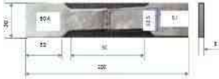
Gambar 7 Standart Specimen Plat Uji Tarik Standart ASME .
