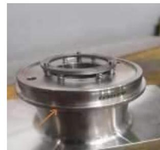
Gambar 3 Mechanical Seal
