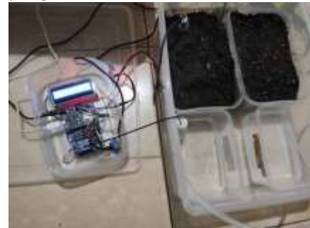
Gambar 7 : Hasil perancangan prototype alat Smart Farming
