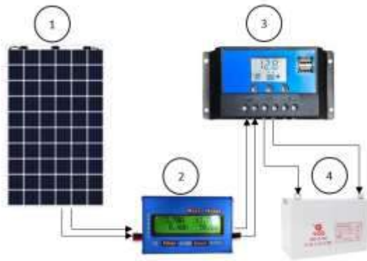
Gambar 3. Wiring Instalasi Panel Surya Sumber Data : Hasil Olahan Data Penelitian
