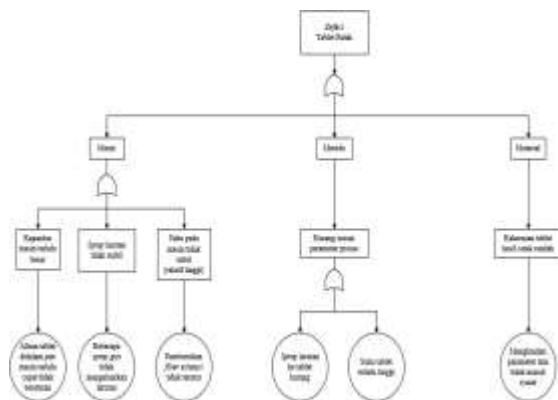
Gambar 2. Analisa Fault Tree Analysis (FTA) Defect Tablet Patah
