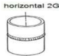
Gambar 2. Posisi pengelasan 2G Sumber: ( https://www.pengelasan.net/posisi-pengelasan by Achmadi)
