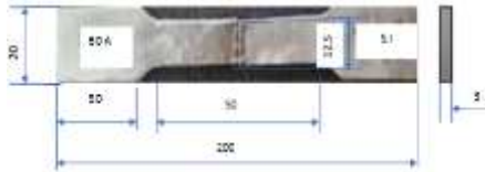
Gambar 7 Standart Specimen Plat Uji Tarik Standart ASME .
