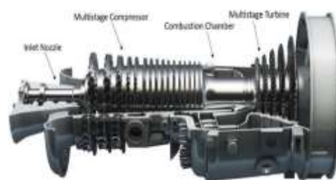
Gambar 1. Turbin Gas GT 2.3 (1) (Sumber: FARR Company & ABB, 1992)
