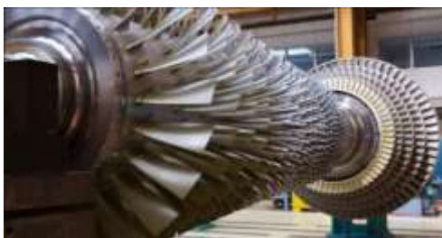
Gambar 3. Photo sudu kompresor (3) (Sumber: Performance Test Codes 10. Compressors and Exhausters. An American national standard , 1997) (3)
