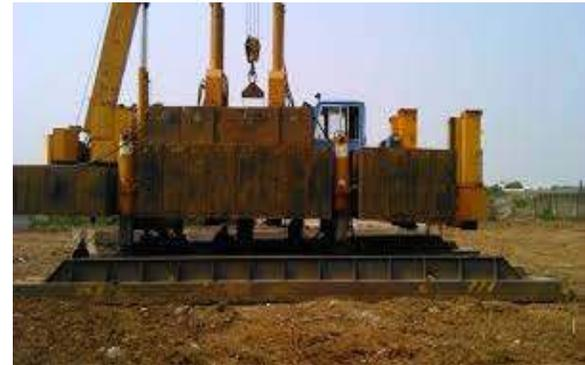
Gambar 3. 2 Hydraulic Static Pile Driving
