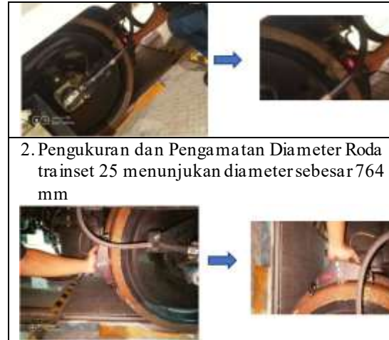
Gambar 6. Data Pengamatan Visual Roda Trainset 25.
