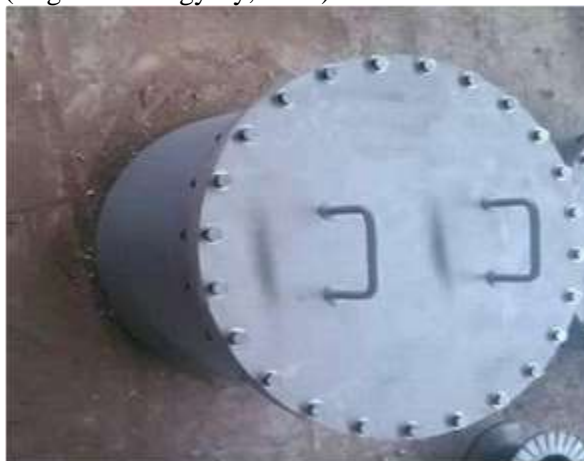
Gambar 6. Man hole (Lobang lalu orang) diameter 10 inc.
